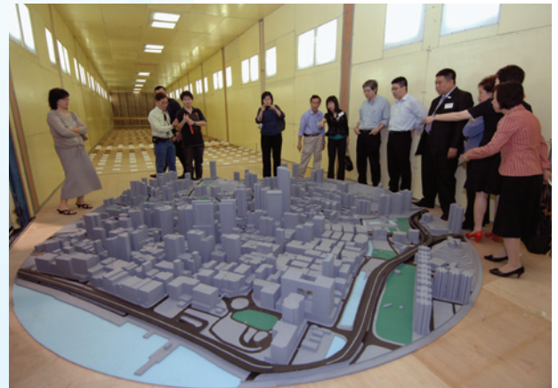
Members of the Kwun Tong District Council observe the wind-tunnel test of the Kwun Tong Town Centre model conducted by the Hong Kong University of Science & Technology.
